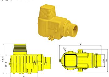
• Junction box for flanged elbow fittings for gas
