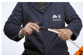
2 Gauge carefully the end of the pipe using the apposite calibrator-countersink art. 3813.
