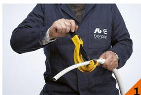
1 Cut perpendicularly the pipe with shears art.3812 avoiding to misshape it.
