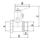
• Water heater safety valve with lever
